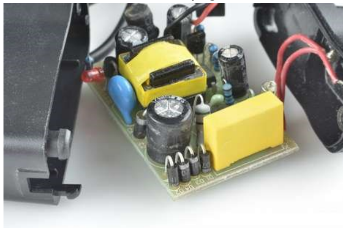
Can you spot the four diodes making a bridge rectifier in this wall wart?
